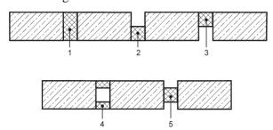
Figure 1 HENSOMASTIK® Acrylic for linear joint and gaps sealing positions
