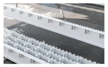
2C steel fire protection systems are mainly applied in the workshop. After a drying time of 24 hours, the coated steel components are optimally protected against mechanical loads and weathering. They can therefore already be stored outdoors and/or transported directly to the site of use and assembled in a time-saving manner.
