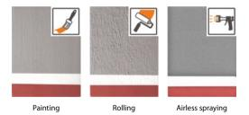
The texture of the final coating is influenced to no little degree by the selected or prescribed application method. A manual application with **brush or roller** gives rise to a heavily textured surface.
