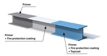
Figure depicts: Coating structure on steel blasted according to Sa 2.5
