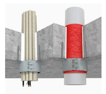
The **HENSOTHERM\* RM 30 / RM 50** for single pipe lead-throughs is used as a sealing of pipes with and without sound insulation as well as EIR / Flex pipes (with and without cables) to restore the fire safety of wall and ceiling constructions that are provided with openings for supply lines. Various common aluminium composite pipes can be laid and sealed as a double feed-through with zero spacing - ideal, for example, for the flow and return of heating installations.
