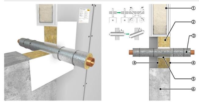
1 = Flexible wall (drywall), 2 = Mineral fiber board 1 x  $\geq$  60 mm, density  $\geq$  150 kg/m<sup>3</sup>, Rockwool Hardrock 040, 3 = Non-combustible metal pipe with stone wool insulation 40 kg/m<sup>3</sup> or higher, 4 = Outer sides coated (DFT  $\geq$  1 mm) with HENSOMASTIK<sup>®</sup> 5 KS Farbe/viskos, circumferential coating,  $\geq$  20 mm width, 5 = Annular gap filled with HENSOMASTIK<sup>®</sup> 5 KS SP (Spachtel), 6 = Rigid wall
