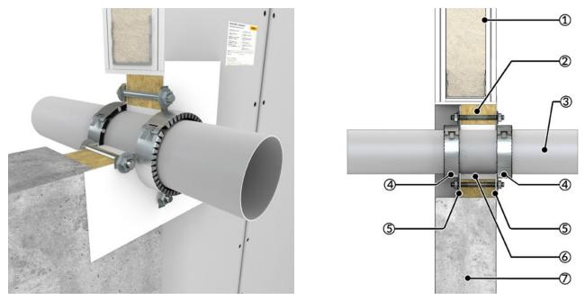
1 = Flexible wall (drywall), 2 = Mineral fiber board 1 x  $\geq$  60 mm, density  $\geq$  150 kg/m<sup>3</sup>, Rockwool Hardrock 040, 3 = Combustible plastic pipe, 4 = HENSOTHERM<sup>®</sup> RM pipe collars fixed with threaded rods M6, nuts and washers (6.4 x 25 mm), 5 = Outer sides coated (DFT  $\geq$  1 mm) with HENSOMASTIK<sup>®</sup> 5 KS Farbe/viskos, circumferential coating  $\geq$  20 mm width, 6 = Annular gap filled with HENSOMASTIK<sup>®</sup> 5 KS SP (Spachtel), 7 = Rigid wall
