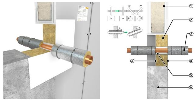
1 = Flexible wall (drywall), 2 = Mineral fiber board 1 x  $\geq$  60 mm, density  $\geq$  150 kg/m<sup>3</sup>, Rockwool Hardrock 040, 3 = Non-combustible metal pipe with stone wool insulation 80 kg/m<sup>3</sup> or higher, 4 = Outer sides coated (DFT  $\geq$  1 mm) with HENSOMASTIK<sup>®</sup> 5 KS Farbe/viskos, circumferential coating  $\geq$  20 mm width, 5 = Annular gap filled with HENSOMASTIK<sup>®</sup> 5 KS SP (Spachtel), 6 = Rigid wall
