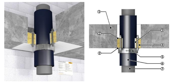
1 = Rigid floor, 2 = Outer sides coated (DFT  $\ge$  1 mm) with HENSOMASTIK<sup>®</sup> 5 KS Farbe/viskos, circumferential coating  $\ge$  20 mm width, 3 = Annular gap filled with HENSOMASTIK<sup>®</sup> 5 KS SP (Spachtel), 4 = Mineral fiber board 1 x  $\ge$  60 mm, density  $\ge$  150 kg/m<sup>3</sup>, Rockwool Hardrock 040, 5 = HENSOTHERM<sup>®</sup> RM pipe collar, secured with M6 threaded rods, nuts and washers 6.4 x 25 mm, 6 = Combustible plastic pipe with sound-insulation mass layer
