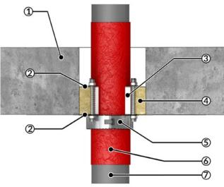
1 = Rigid floor, 2 = Outer sides coated (DFT  $\geq$  1 mm) with HENSOMASTIK<sup>®</sup> 5 KS Farbe/viskos, circumferential coating  $\geq$  20 mm width, 3 = Annular gap filled with HENSOMASTIK<sup>®</sup> 5 KS SP (Spachtel), 4 = Mineral fiber board 1 x  $\geq$  60 mm, density  $\geq$  150 kg/m<sup>3</sup>, Rockwool Hardrock 040, 5 = HENSOTHERM<sup>®</sup> RM pipe collar, secured with M6 threaded rods, nuts and washers 6.4 x 25 mm, 6 = Combustible plastic pipe with, PE-foam sound decoupling
