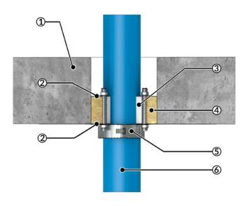
1 = Rigid floor, 2 = Outer sides coated (DFT  $\ge$  1 mm) with HENSOMASTIK<sup>®</sup> 5 KS Farbe/viskos, circumferential coating  $\ge$  20 mm width, 3 = Annular gap filled with HENSOMASTIK<sup>®</sup> 5 KS SP (Spachtel), 4 = Mineral fiber board 1 x  $\ge$  60 mm, density  $\ge$  150 kg/m<sup>3</sup>, Rockwool Hardrock 040, 5 = HENSOTHERM<sup>®</sup> RM pipe collar, secured with M6 threaded rods, nuts and washers 6.4 x 25 mm, 6 = Combustible plastic pipe
