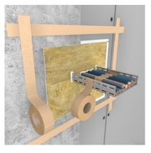
Apply duct tape for a min. 20 mm wide circumferential coating.
