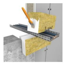
Apply thick layer of **HENSOMASTIK<sup>®</sup> 5 KS Farbe /viskos** to butter all cut edges and the outer edges oft he mineral fibre board.
