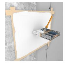
Apply **HENSOMASTIK<sup>®</sup> 5 KS Farbe/viskos** to the mineral fibre boards and 20 mm wide (DFT ≥ 1 mm) all round.
