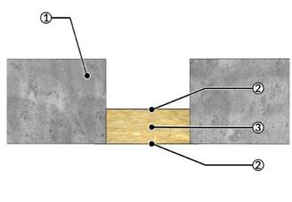
1 = Rigid floor, 2 = Outer sides coated (DFT  $\ge$  1 mm) with HENSOMASTIK<sup>®</sup> 5 KS Farbe/viskos, circumferential coating  $\ge$  20 mm width, 3 = Mineral fiber board 1 x  $\ge$  60 mm, density  $\ge$  150 kg/m<sup>3</sup>, Rockwool Hardrock 040
