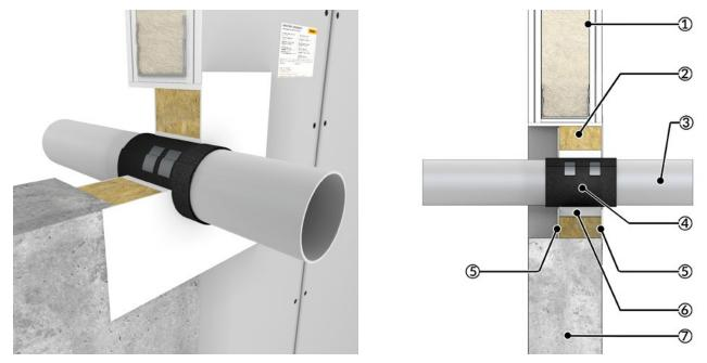
1 = Flexible wall (drywall), 2 = Mineral fiber board 1 x  $\geq$  60 mm, density  $\geq$  150 kg/m<sup>3</sup>, Rockwool Hardrock 040, 3 = Combustible plastic pipe, 4 = HENSOTHERM<sup>®</sup> 7 KS Gewebe 100, fixed with adhesive tape or metal straps or wires  $\geq$  0.6 mm, 5 = Outer sides coated (DFT  $\geq$  1 mm) with HENSOMASTIK<sup>®</sup> 5 KS Farbe/viskos, circumferential coating  $\geq$  20 mm width, 6 = Annular gap filled with HENSOMASTIK<sup>®</sup> 5 KS SP (Spachtel), 7 = Rigid wall
