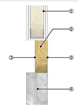
1 = Flexible wall (drywall), 2 = Mineral fiber board 1 x  $\ge$  60 mm, density  $\ge$  150 kg/m<sup>3</sup>, Rockwool Hardrock 040, 3 = Outer sides coated (DFT  $\ge$  1 mm) with HENSOMASTIK<sup>®</sup> 5 KS Farbe/viskos, circumferential coating  $\ge$  20 mm width, 4 = Rigid wall
