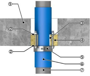
1 = Rigid floor, 2 = Outer sides coated (DFT  $\geq$  1 mm) with HENSOMASTIK<sup>®</sup> 5 KS Farbe/viskos, circumferential coating  $\geq$  20 mm width, 3 = Annular gap filled with HENSOMASTIK<sup>®</sup> 5 KS SP (Spachtel), 4 = Mineral fiber board 1 x  $\geq$  60 mm, density  $\geq$  150 kg/m<sup>3</sup>, Rockwool Hardrock 040, 5 = HENSOTHERM<sup>®</sup> RM pipe collar, secured with M6 threaded rods, nuts and washers 6.4 x 25 mm, 6 = Combustible plastic pipe with FEF-insulation (CS)
