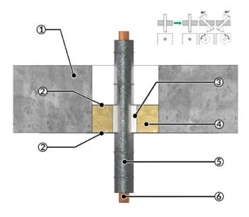
1 = Rigid floor, 2 = Outer sides coated (DFT  $\ge$  1 mm) with HENSOMASTIK<sup>®</sup> 5 KS Farbe/viskos, circumferential coating  $\ge$  20 mm width, 3 = Annular gap filled with HENSOMASTIK<sup>®</sup> 5 KS SP (Spachtel), 4 = Mineral fiber board 1 x  $\ge$  60 mm, density  $\ge$  150 kg/m<sup>3</sup>, Rockwool Hardrock 040, 5 = Stone wool insulation 80 kg/m<sup>3</sup> or higher, 6 = Non-combustible metal pipe
