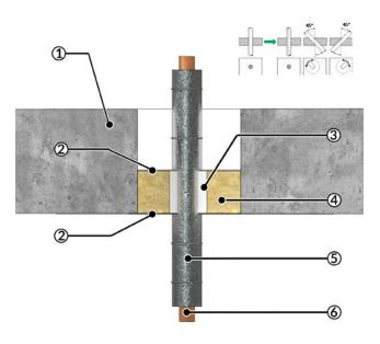
1 = Rigid floor, 2 = Outer sides coated (DFT  $\geq$  1 mm) with HENSOMASTIK<sup>®</sup> 5 KS Farbe/viskos, circumferential coating  $\geq$  20 mm width, 3 = Annular gap filled with HENSOMASTIK<sup>®</sup> 5 KS SP (Spachtel), 4 = Mineral fiber board 1 x  $\geq$  60 mm, density  $\geq$  150 kg/m<sup>3</sup>, Rockwool Hardrock 040, 5 = Stone wool insulation 40 kg/m<sup>3</sup> or higher, 6 = Non-combustible metal pipe
