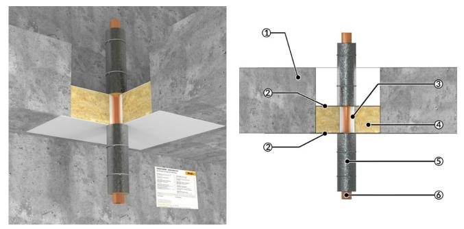
1 = Rigid floor, 2 = Outer sides coated (DFT  $\ge$  1 mm) with HENSOMASTIK<sup>®</sup> 5 KS Farbe/viskos, circumferential coating  $\ge$  20 mm width, 3 = Annular gap filled with HENSOMASTIK<sup>®</sup> 5 KS SP (Spachtel), 4 = Mineral fiber board 1 x  $\ge$  60 mm, density  $\ge$  150 kg/m<sup>3</sup>, Rockwool Hardrock 040, 5 = Stone wool insulation 80 kg/m<sup>3</sup> or higher, 6 = Non-combustible metal pipe
