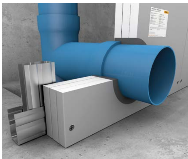
(1) Steel stud frame (2) At least three layers of at least 15 mm-thick type DF plasterboards according to EN 15283-1 (3) Combustible pipe with or without pipe connection inside the wall (4) Annular gap filled with HENSOTHERM® 7 KS viskos (5) Solid floor
