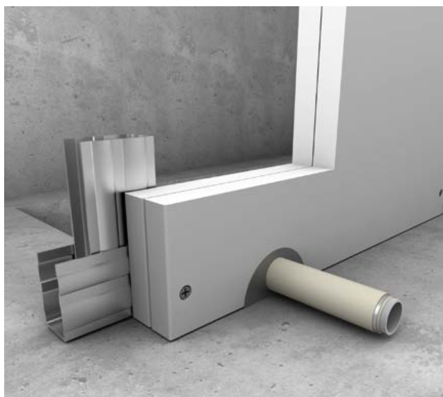
(1) Steel stud frame (2) At least two layers of at least 20 mm-thick type GM-F plasterboards according to EN 15283-1 (3) Annular gap filled with HENSOTHERM® 7 viskos (4) Aluminium composite pipe, individually or in series with zero spacing (5) Solid floor
