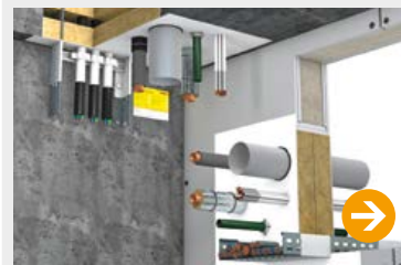
HENSOMASTIK® Mixed Penetration Seal EI 90/EI 120 Mixed soft penetration seal | ETA 20/1309
