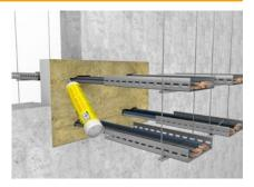
→ Fill the annular gap between cables and mineral fibre board with HENSOTHERM® 7 KS viskos to a depth of at least 25 mm
