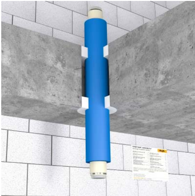
1 = Rigid floor, 2 = Annular gap (width 10–20 mm) filled \geq 25 mm deep with HENSOMASTIK® Acrylic, optional backing with stone wool (class A1 or A2 according to EN 13501-1), 3 = Insulation, 4 = Aluminium-composite pipe
