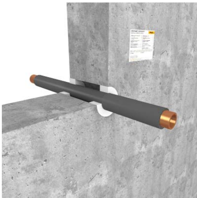
1 = Rigid wall, 2 = Annular gap (width 10–20mm) filled \geq 25 mm deep with HENSOMASTIK® Acrylic, optional backing with stone wool (class A1 or A2 according to EN 13501-1), 3 = Non-combustible metal pipe, 4 = Insulation
